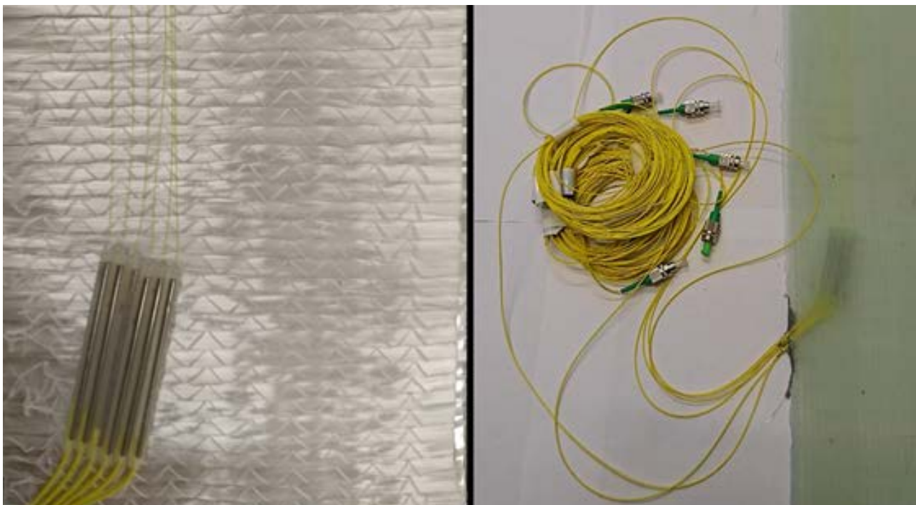
Instrumentation of GFRP laminate before and after vacuum infusion. As can be seen, the optical fibers are embedded inside the laminate and the picture to the left is from ply number two out of four, meaning the fibers are located in the middle of the laminate.
